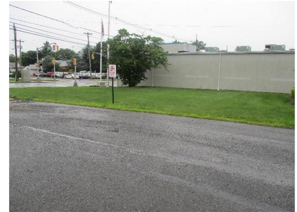
Runoff can be captured and treated by replacing the existing parking spaces with porous pavement. The site drains to an existing turf grass area to the east where a rain garden can be installed to filter and infiltrate stormwater runoff. A preliminary soil assessment suggests that the soils have suitable drainage characteristics for green infrastructure.
