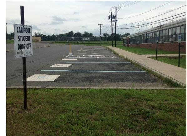
Parking spaces south of the school can be replaced with pervious pavement to capture and infiltrate stormwater. A bioretention system can be installed to capture, treat, and infiltrate rooftop runoff. A preliminary soil assessment suggests that the soils have suitable drainage characteristics for green infrastructure.
