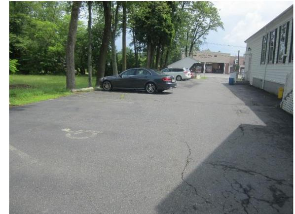
Parking spaces north of the church can be replaced with pervious pavement to capture and infiltrate stormwater. A bioretention system can be installed to capture, treat, and infiltrate roof runoff from the church. A preliminary soil assessment suggests that more soil testing would be required before determining the soil's suitability for green infrastructure.
